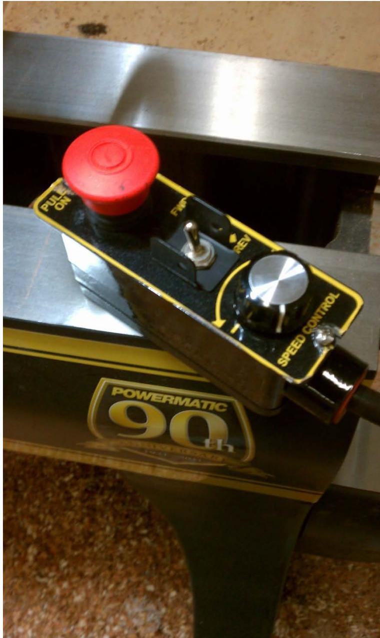
The remote switch. It sticks in the horizontal position better than in the vertical position due to the curved sides of the lathe ways.
