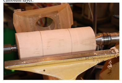
Measure the diameter and put 2 lines this distance apart on the cylinder. Use a parting tool to cut down at these lines and the use the rough out gouge to remove the wood outside these marks.
