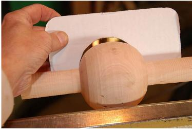
Use a parting tool to cut the tenons smaller outside the ball.
