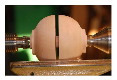
Remove this from the lathe and cut it in half with a handsaw. If the tenon is small enough you may be able to simply twist the two apart. You now have 2 side grain bowls.
