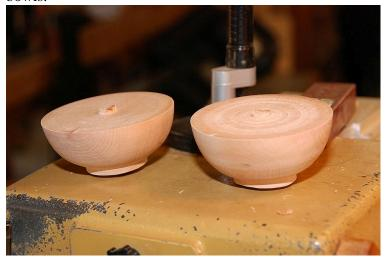
Mount a faceplate with a waste piece of wood on the lathe and turn a small hole for the little tenon on the bowl bottom. Then glue the bowl into the wasteblock.
