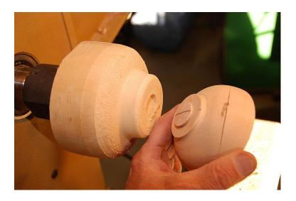
Turn the inside of the bowl. You may need to true up the outside as well. Sand the bowl inside and out. Use a parting tool to cut the bottom of the bowl. Now turn an opening in the waste block the size of the bowl. Insert the bowl into this opening and bring the tailstock up to hold it. If it doesn't fit snuggly use paper towels to make if fit more
