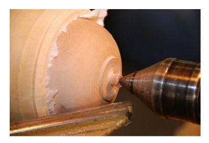
You can now carve this little tenon off. I use my spindle gouge to remove the little tenon. I push forward very gently while keeping pressure on the bevel to hold the bowl in place. This allows me to cut allof the tenon off with the spindle gouge instead of carving it off. Sand this area.
