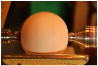
Turn away the shadow potion. Now imagine 2 bowls facing each other. Use a parting tool to make a shallow cut to help identify the bowls. Turn the outside of each bowl shape including the foot and a small tenon. Sand the outside of the bowls. Now use the parting tool to extend the center cut down until there is a very small tenon.
