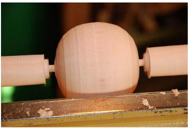
Draw a line at the center of the ball. Then remove ball from the lathe and cut the tenons off. Now mount the ball between centers using the line as your center marks. Now the pith runs perpendicular to the bed. Rotate the ball by hand and check to see that it's centered. If not readjust it slightly. Your ball probably won't be round at this point. You can see a shadow as it rotates.
