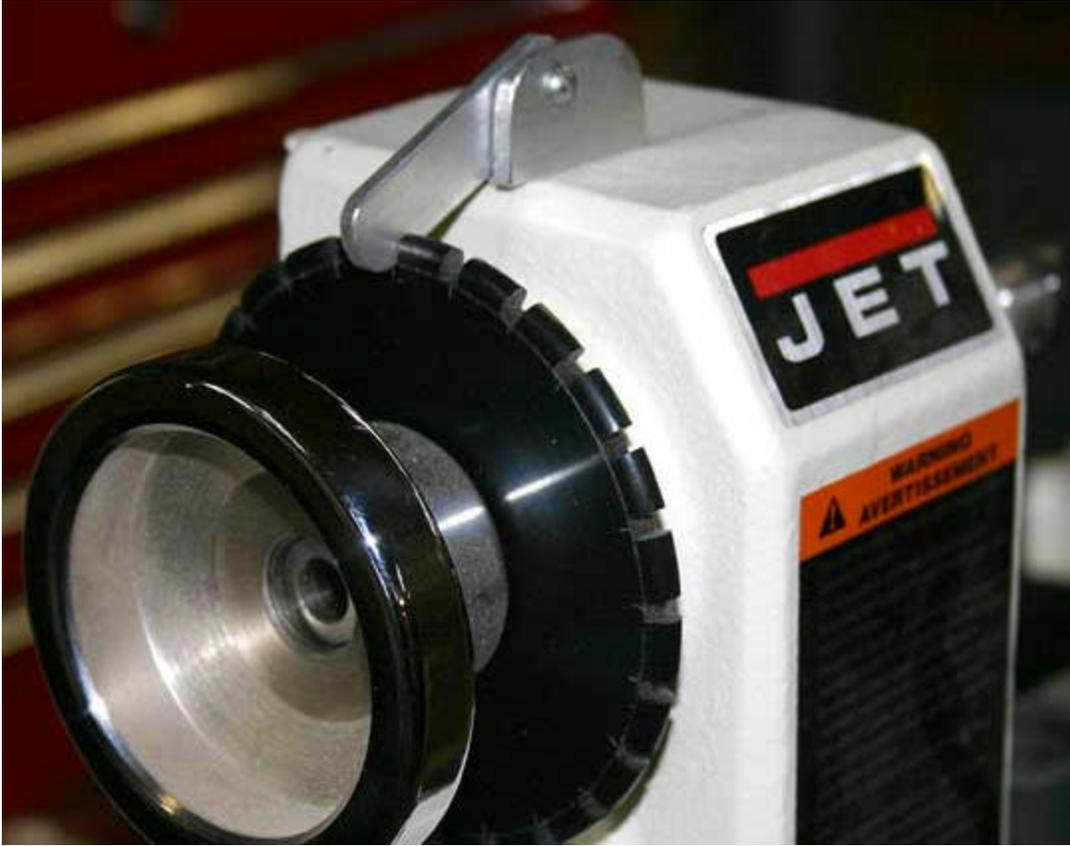
I've also built and installed a locking index wheel that uses round drilled holes. The inner pin is spring loaded. The wheel was easier to build but the internal mechanism was complicated to make it work smoothly. An easier method would be to glue a flat block between the index wheel and the headstock and drill one hole to match the index wheel. Then just use a pin that is inserted from the backside. If you put a rare earth magnet on the lathe you will have a good place to store the pin.
