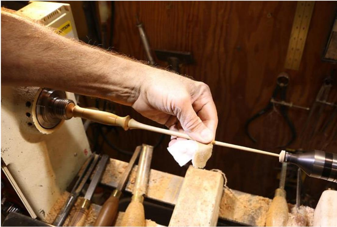
I like to use beeswax to finish cedar wands, applied with the lathe running and melted into the surface with friction from a small piece of cloth.
