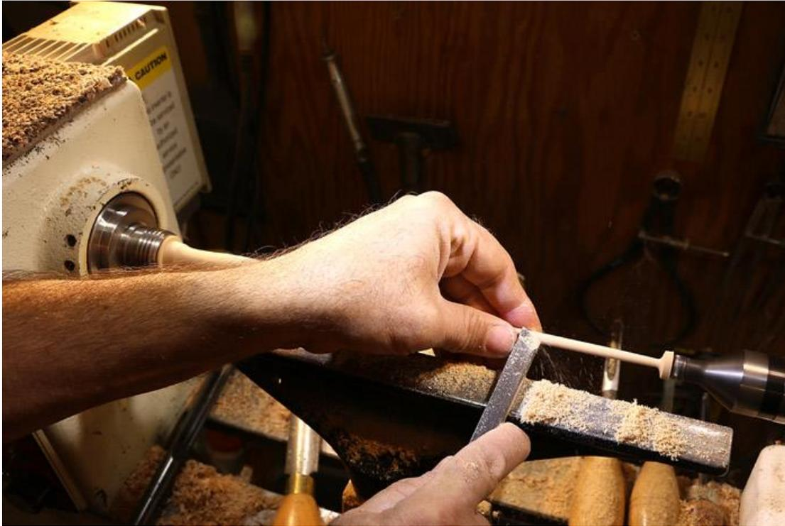
This, of course, requires holding the tool with the right hand only. I grip very near the tip and support the end of the handle by forcing it against the underside of my forearm. This supports the tool well.
