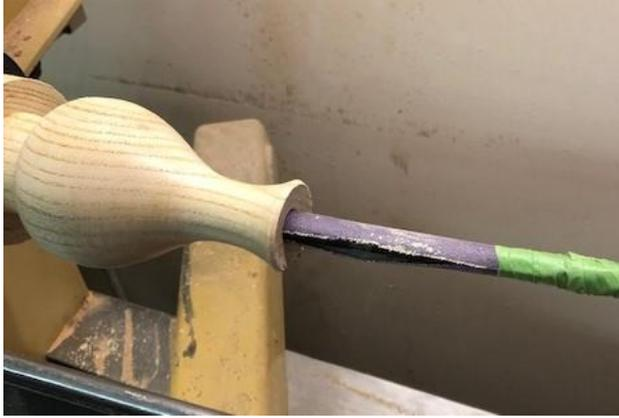
**5. Measure the depth of the hole and determine where the bottom of the bud vase will be. Use a parting tool to make a 1/2" deep cut to show you where the bottom will be when shaping the bud vase.**
