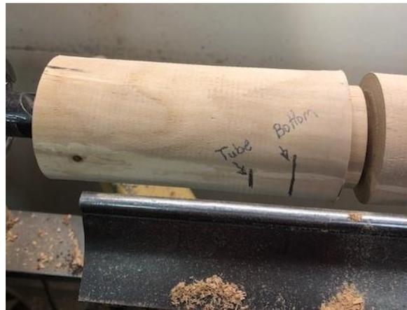
**3. Remove and re-mount the wood into the chuck. Begin shaping the top and make a starter hole for the 1/2" drill bit. Put drill chuck in the tail stock and drill a 1/2" hole as deep as the glass test tube is long. About 5" normally. I like to leave about 1/8" of the tube sticking out of the hole when finished.**
