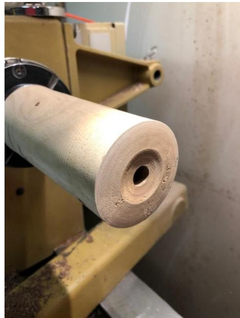
**4. Using a sanding stick, sand the inside of the drilled hole until the test tube slides in easily. If you have a 9/16" drill bit, then the sanding stick will not be required. But always check to make sure the glass test tube will easily go into the drilled hole with no pressure.**
