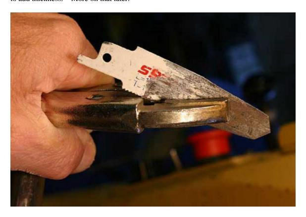
To use the tool simply clamp it in a pair if vise grips. Extend the tip out about an inch. More extension makes the tool vibrate slower. Less extension makes it vibrate faster. The faster it vibrates the closer the chatter work marks are together.
