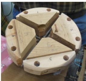
Homemade wooden jaws to hold the globe for drilling and hollowing
