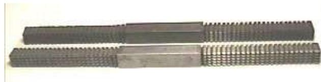
The rethreading tools I have (see above image) allow for cutting 9, 10, 11, 12, 13, 14, 16, 18, 20, 24, 27, 28, and 32 threads per inch. That is a pretty good assortment.
