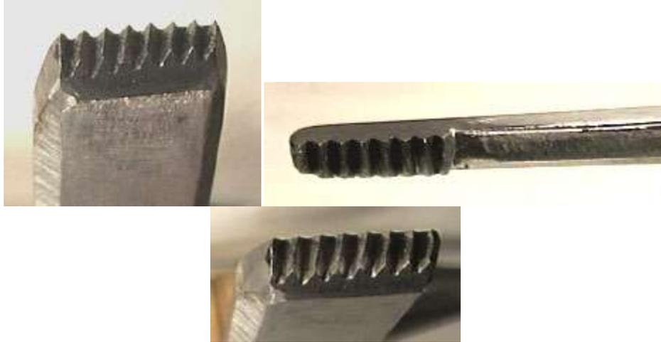
The slant required varies with the diameter of the wood on to which the threads are to be cut. I slanted mine based upon the slant of a standard threaded bolt of the size I wanted to duplicate. In addition to producing tighter fitting threads in the finished product, this slant in the cutters tends to almost automatically feed the chaser into the wood at the correct speed and to help avoid cross-threading.
