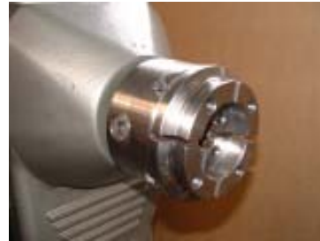
The Supernova 2 chuck on Nova 3000 DVR lathe
